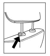
Pull the head restraint up to raise it. To lower the head restraint, press the button, located on the top of the seatback, and push the head restraint down.
